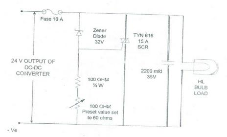
Whenever output voltage shoots up due to MOSFET failure, the same will exceed the Zener knee voltage(33V) resulting puncture of Zener junction due to which Zener develops SCR gate trigger voltage(30V) with the help of preset threshold resistor. This causes turning'ON' of SCR resulting in flow of short circuiting current through the output of DC-Dc converter and isolate the HL lamp load.
